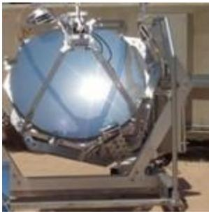
[Distributed Solar Power](#): Israel-based firm developing a CPV/CHP system that produces electricity and heat using sun-tracking miniature PV concentrators. The system has a claimed ~75 percent efficiency and is intended for on-grid customers. It can produce high quality heat for steam generation, cooling and AC (using absorption cooling), space and water heating, and process heat. The firm is working with Italy's [Shap](#) and has raised \$1.2 million from Israel's Aurum Ventures et al.
